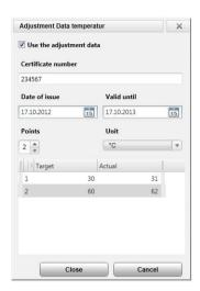
Once the calibration data has been entered, this is stored in the probe permanently. The probe takes deviations into account automatically during measurement, thereby generating a zero-error display.
