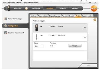
The probe name of any connected probe can be changed and calibration data from the calibration protocol stored in the probe.
